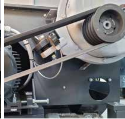
V-belt drive with gearbox limit switch
