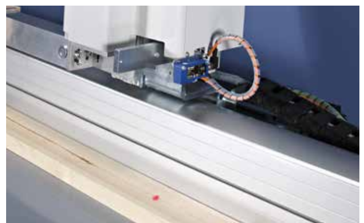
Close-up of pusher with workpiece measurement sensor
