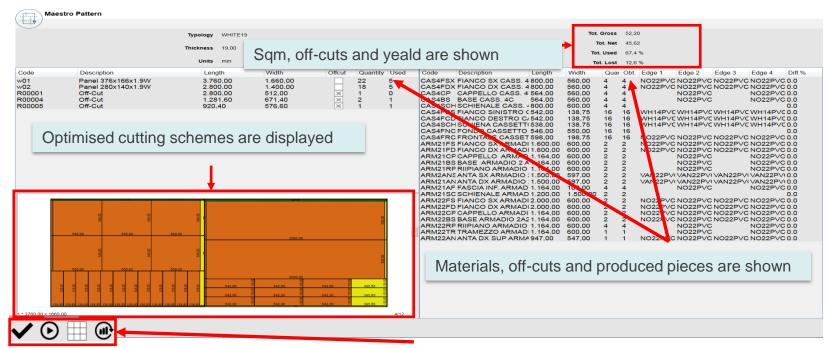
Selecting the appropriate buttons is possible to generate directly the machine programs for Maestro Cut, sending of cutting programs to the machine, displaying all cutting schemes and updating the material stock (useful for weekly/monthly plan).
