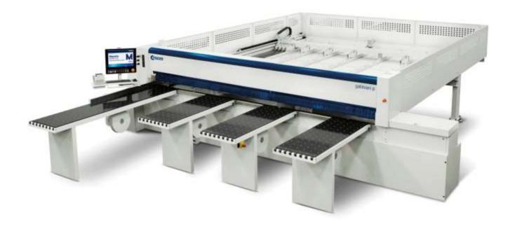
**gabbiani p** automatic single blade beam saw born to be at the forefront. The unique entry level machine having all the features of a top range one.
