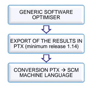
Maestro converter cut is the module that allows to integrate any type of cutting optimization programs with SCM beam saws through PTX file (minimum release 1.14).
