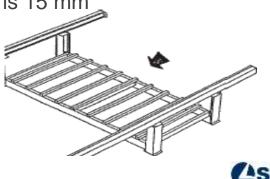
Fixed air floating table with feeding rollers  $(1500 - 2500 - 3000 \times 600/800 \text{ mm})$ Mobile air floating table with feeding rollers  $(1500 - 2500 - 3000 \times 600 \text{ mm})$
