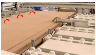
• The auxiliary pusher, with counter sensor, pushes the stack panels against the open grippers of the clamps in the main pusher
