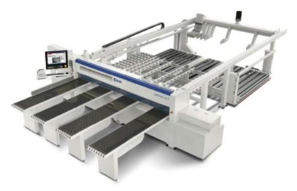
**gabbiani gt 2** high performance automatic single blade beam saw for the quality of its cut finishing and working speed, in order to satisfy all the production requirements of the furniture enterprises.
