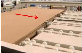
The stop-pack devices block the stack on the elevator table to avoid the load of the underlying panels.
