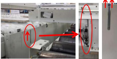
• For thin panels stacks the locking device is deactivated to allow the loading of panels stacks showing marked geometric irregularity
