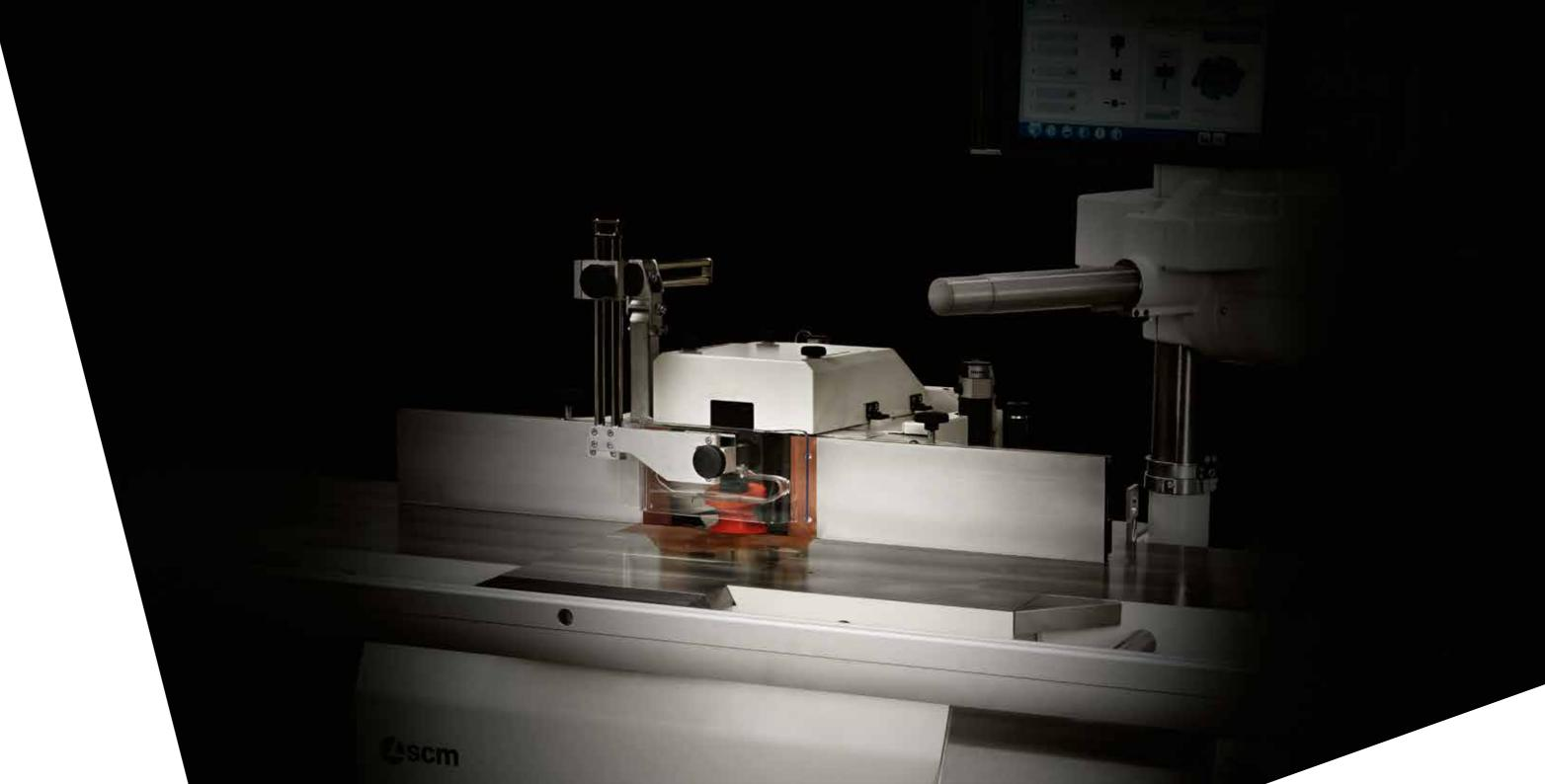
Speed of setting-up due to the unique movement mechanism of the spindle (SCM patent), which allows the operator to position independently the height of the tool with the tilted spindle and the moulder fence. Maximum performance using the latest technology of the screws with recirculating ball-bearings and the linear guides which guarantee a total absence of vibration and wear, therefore much reduced maintenance (centralised lubrication).
