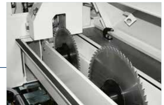
SAW-SET: tool changing has never been so easy. Fast and precise tools adjustment due to the electronic setting (opt.).
