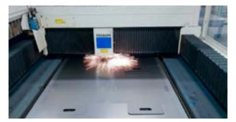
Steel plate laser cutting
