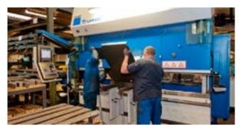
Computer assisted steel plate bending
