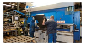
Computer assisted steel plate bending
