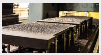
Surface scraping of cast iron table
