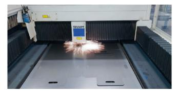
Steel plate laser cutting
