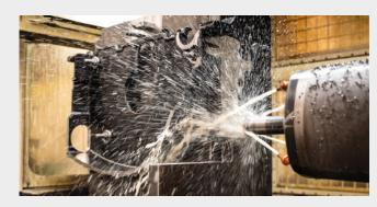
CNC Machining of cast iron saw aggregate
