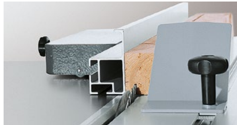
Set the height of the blade and the width on the rip fence.
