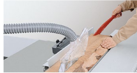
Guide the workpiece along the rip fence and over the rotating saw blade, using the push stick if necessary.
