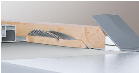
Fix the workpiece under the clamping shoe and cut the chamfer.
