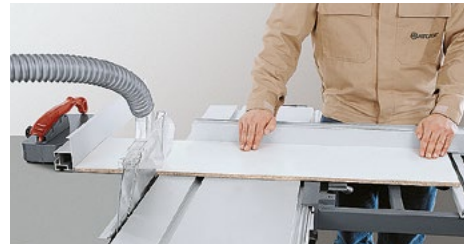
Cut panel strips to final length on the rip fence.
