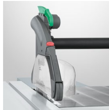
The optional big extraction hood ensures even more work safety and better handling of angle cuts. The hood can be adjusted to the respective material thickness steplessly and self-locking. The scope of delivery includes a narrow hood for 90° cuts and a wide hood for mitre cuts.
