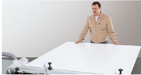
Align the panel and make a trim cut.
