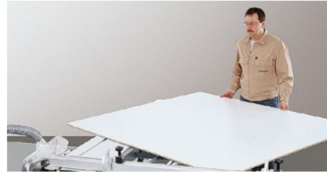
Turn the panel anti-clockwise and place the trimmed edge against the fence.
