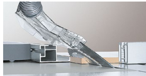
Bevel ripping on the rip fence with workpiece on the sliding table.
