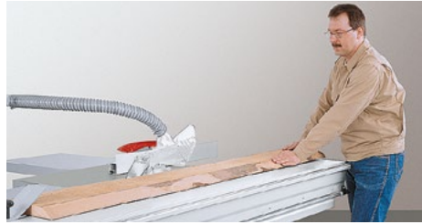
Align and trim the material along the cutting line.
